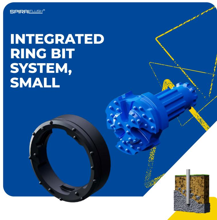
Integrated ring bit systems, divided into small and large designs, are designed for drilling end-bearing piles through overburden into bedrock. The system can drill straight and inclined piles through boulders and rock layers and it easily manages situations where the bedrock itself is inclined.
